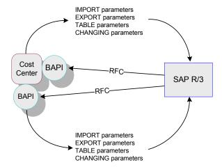
The meta data for a BAPI/RFC in SAP R/3 is extracted by the BAPI wizard, which uses it to build the BAPI/RFC OTD. This OTD is used in Java Collaborations and eInsight Business Processes to invoke or receive the BAPI/RFC call.
